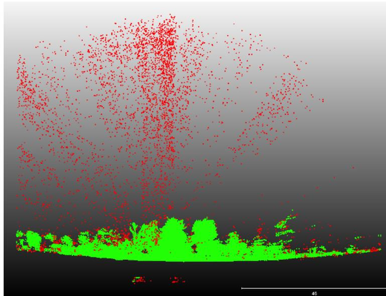
**Figure 6.6:** A 2 m deep cross section of a subplot point cloud showing the efficacy of the noise reduction and voxelisation process. Red points are excluded by the process, while green points are preserved for further analysis.
