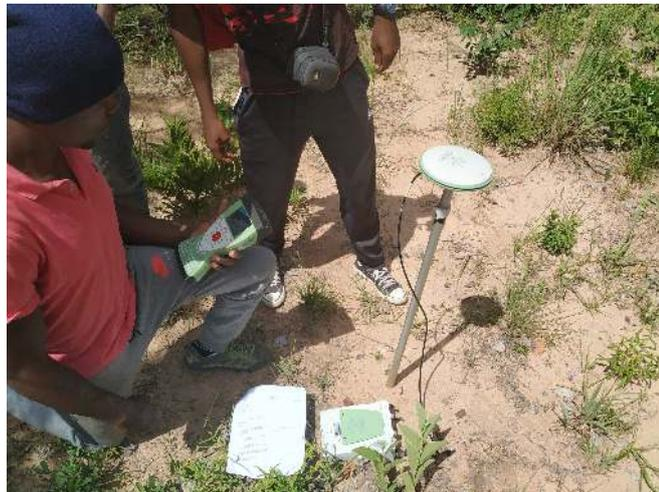
**Figure 6.3:** A Leica VIVA GS10 GNSS unit in the field, showing the antenna atop an aluminium pole, attached to the base station on the ground, and the rover terminal in the hand of a research assistant.
