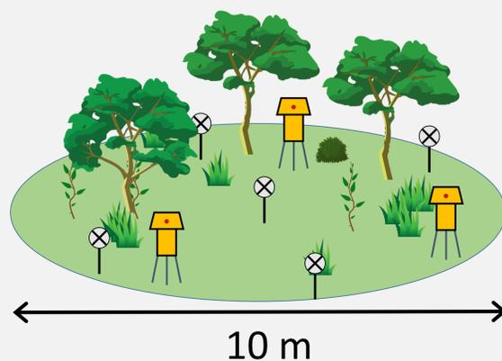
A Leica HDS6100 Phase Shift Terrestrial Laser Scanner (TLS) was used to construct 3D shadowless images of the foliage inside each subplot. Reflective targets were used to allow the data to be compared with satellite LiDAR products in the future, greatly extending the value of the data.
